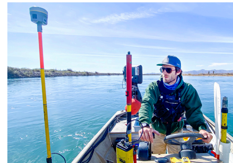
Vessel "SeaArk" surveying the Colorado River with the Trimble R12i, Trimble RTX and TSC7 controller.
