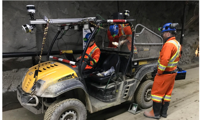
The Applanix navigation system on a subterranean transport vehicle, with front- and back-facing LiDAR to mitigate self-occlusion, and vertically-mounted LiDAR for mapping. The integrated POS LV provides inertial measurements and time-synchronization between all sensors.
