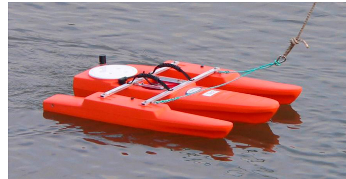
Tethered float and ADCP used for previous surveys
