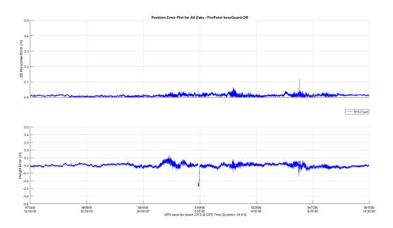
With lonoGuard enabled, the ProPoint RTK solution sees only a slight increase in noise during the peaks of the storm, but overall positioning is improved and outliers are removed.
