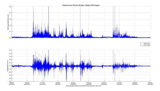
The Trimble ProPoint engine (without lonoGuard) performs better, although it struggles to provide reliable positioning with errors of tens of centimeters.<sup>1</sup>
