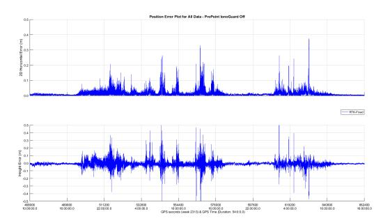
Conversely, a GNSS receiver on the same antenna running lonoGuard technology reflects a dramatic improvement in positioning performance.
