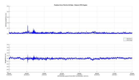
The Trimble ProPoint engine (without IonoGuard) performs very well during the storm, showing a significant improvement over the historic RTK engine.
