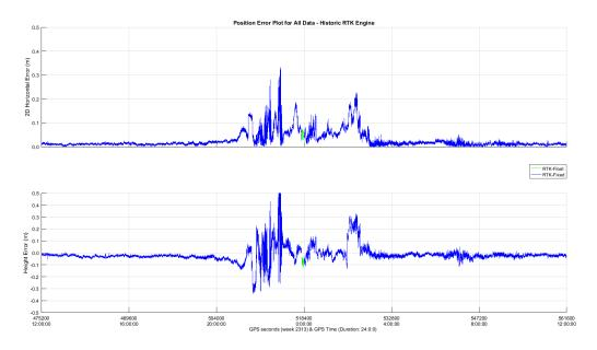
The new Trimble ProPoint engine (without lonoGuard) performed considerably better; however, additional noise and an almost 30 centimeter outlier in the vertical was observed.
