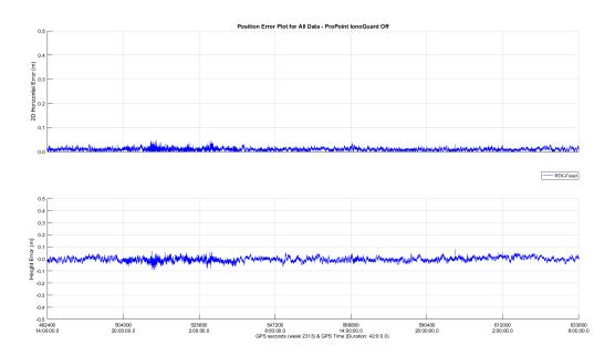
With lonoGuard enabled, the ProPoint RTK solution shows only slight improvements, indicating that the effects of the storm at mid-latitudes in Europe were minimal during this specific event.
