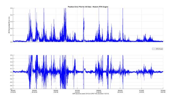
The Trimble ProPoint engine (without lonoGuard) performs better, although it struggles to provide reliable positioning with errors of tens of centimeters and occasionally drops out of RTK-fixed state.
