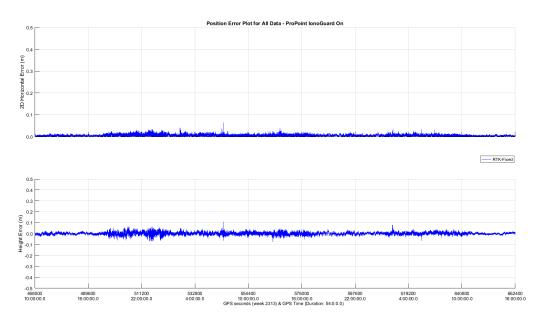
Some limited impact is seen from the ionospheric disturbance; however, users in areas affected by scintillation and other disturbances reported being able to work through any issues using lonoGuard, while other machines were forced to stop due to positioning inaccuracies.
