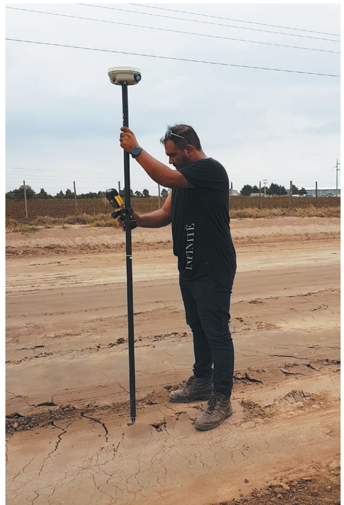
A DBA topographer highlights ground points on the study trace to generate basic engineering plans.
