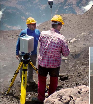
Researchers use Trimble GNSS to locate aerial photo targets and gravimetry points.
