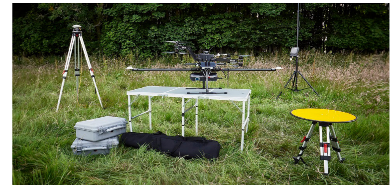
The complete Routescene UAV LiDAR system
