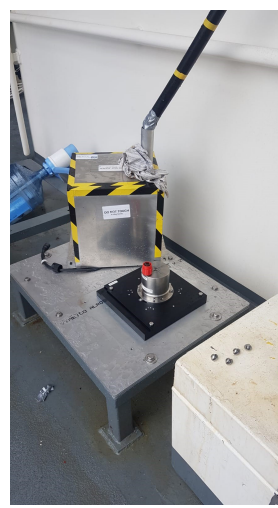
Figure 2: Applanix IMU mounting location with protective covering and cable routing solution
