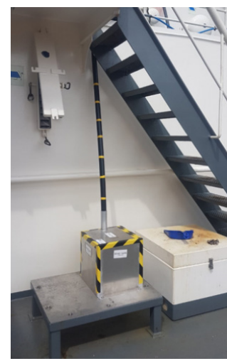
Figure 2: Applanix IMU mounting location with protective covering and cable routing solution
