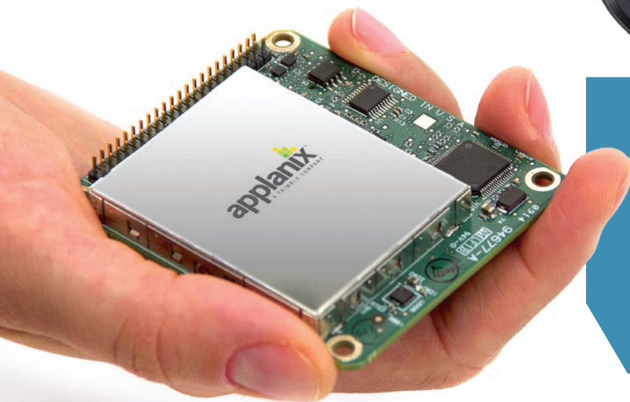
APX-15 UAV – Survey-grade GNSS and MEMS inertial sensors on a single board.
