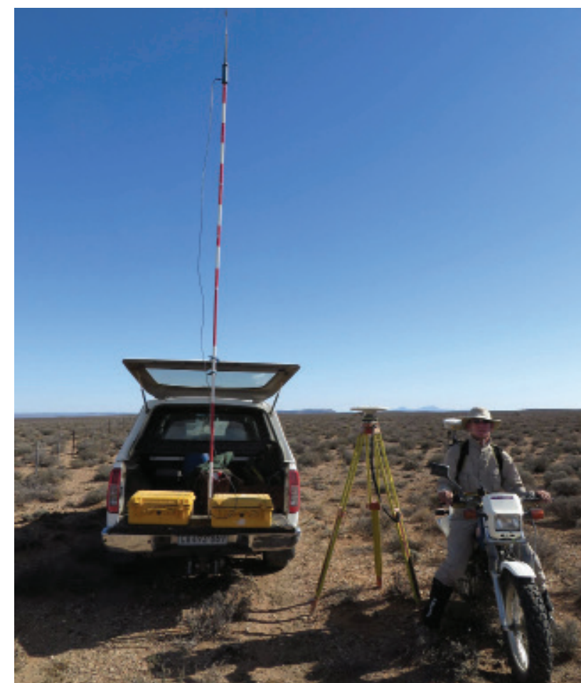
Initial surveys in 2014 required multiple RTK base stations and radio transmitters.
