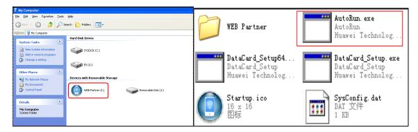
4. If the drive path **Web Partner** not showing up, make sure there is no damage on USB cable and no contamination at PC USB connectors. Try to re-plug in USB connectors (both end of USB cable) to E8372h and computer again.
