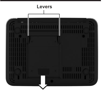
To remove the Hard Drive from the VIP5662W, perform the following procedure.
