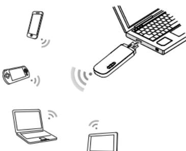
**Scenario 3: Multi-device Internet access using Wi-Fi (connected to the power adapter)**
