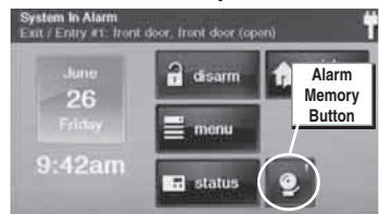
Security Screen with Alarm Memory Button
