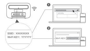
Once the router has connected to a mobile data network, you can connect your computer or mobile phone to the router's Wi-Fi network to access the Internet. Please refer to the label on the back of the router for the default wireless network name (**SSID**) and password (**Wi-Fi KEY**).
