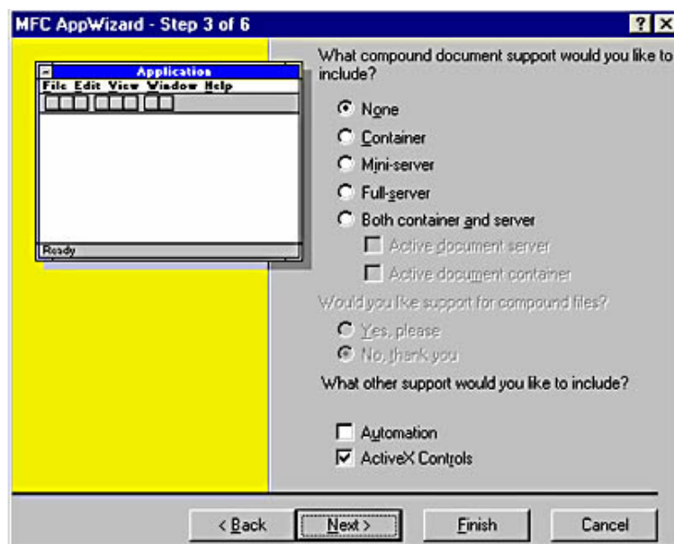
Figure 21-23. Checking AppWizard's ActiveX Controls box makes any MFC dialog an ActiveX control container.
