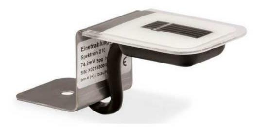
This sensor is used to measure irradiated energy and is normally attached to the module frame. Comparing the irradiated power to the inverter power provides a simple indicator as to whether the PV system is working properly.
