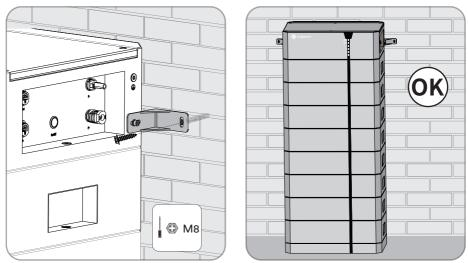
Step 10: Secure the hanger using screws(M8×40).
