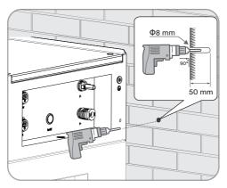
Insert a screw anchor into the hole. Repeat on the other side of the BCU. Step 8:
