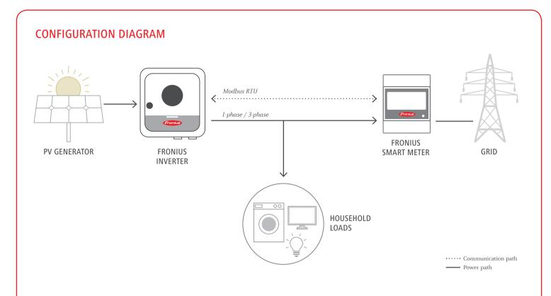
The Fronius Smart Meter is compatible with all inverters with an RS485 interface (Modbus RTU). The Fronius Smart Meter can be retrofitted at any time together with the Fronius Datamanager 2.0 in inverters that have already been installed.
