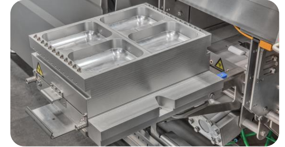
Quick tooling exchange of bottom tool from the side
