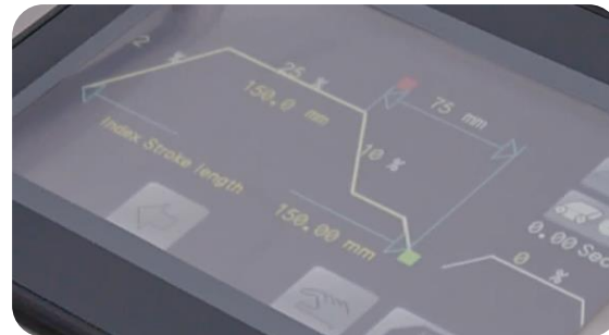
Servo-driven chain: optimal, adjustable transport curve, even for liquids
