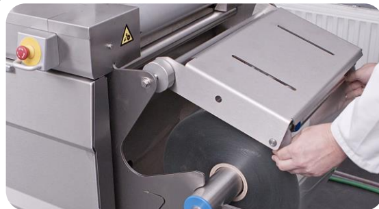
Film support on both sides: precise, stable → no wrinkles, perfect shape
