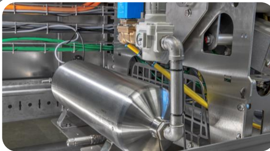
Vacuum pump up to 300 m 3 can be integrated
