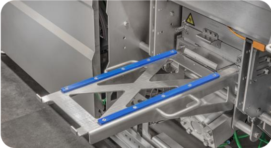
Quick tooling exchange of bottom tool from the side
