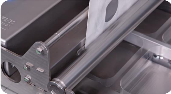
Photo cell and perfectly placed film brake for optimal positioning
