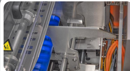
Removable pistons, easy exchange to different tracks
