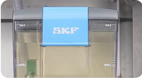
Automatic lubrication of chain
