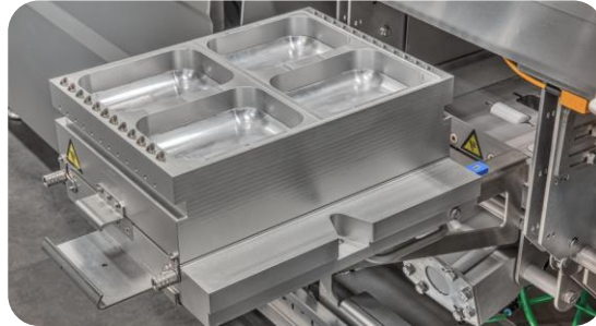
Quick tooling exchange of bottom tool from the side
