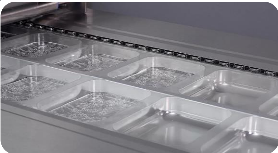
Servo-driven chain: optimal, adjustable transport curve, even for liquids
