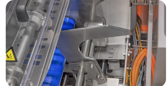
Removable pistons, easy exchange to different tracks
