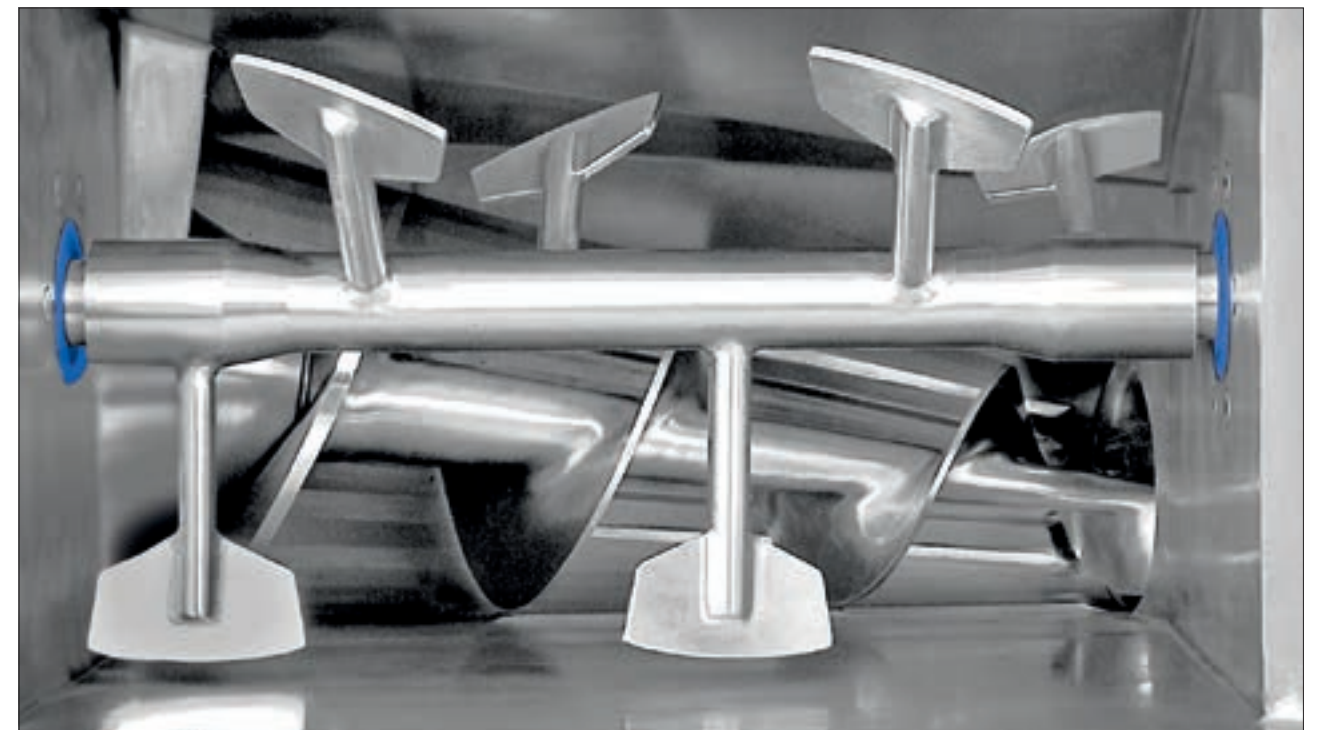
Automatic Mixing Grinder with mixing paddles
