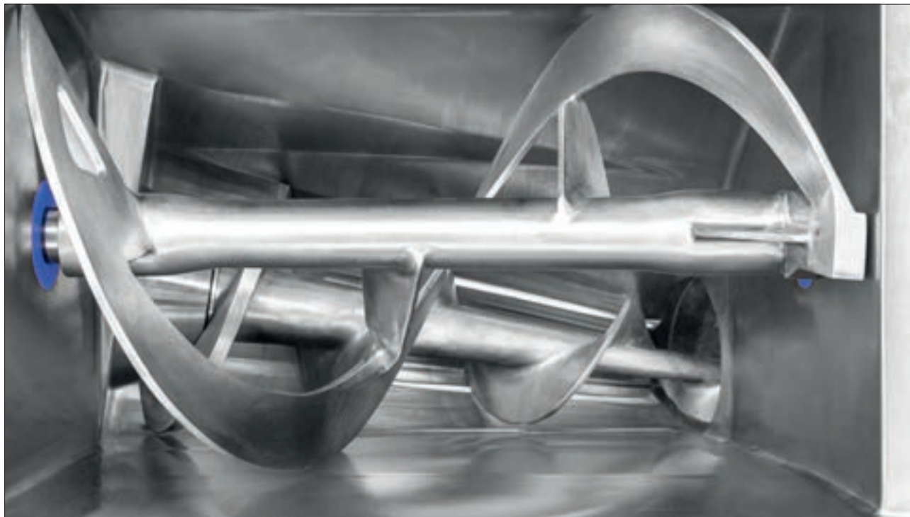
Automatic Mixing Grinder with mixing spiral
