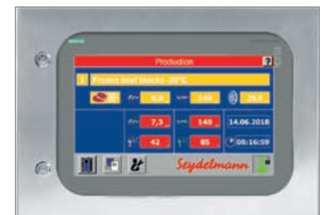
Command 700 W: Automatic regulation of the feeding speed
