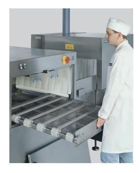
Easy and fast cleaning — the complete conveyor belt can be pulled from the BL15 in a few steps — drip tray and the inside of the machine are freely accessible.
