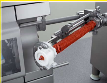
Casing brake assistant - semi-automatic casing brake holder system
