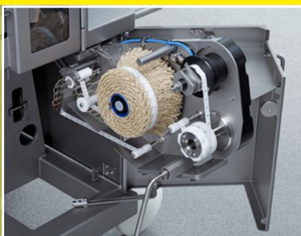
Retractable automatic looper GSA for easy reloading of loops
