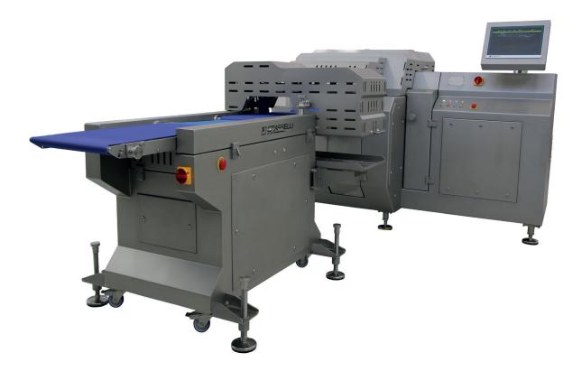
**KSL PC line** is a **weight control automatic horizontal slicer** capable of dynamically adjusting slice thickness through blade positioning to obtain **equal weight portions of slices**. This is achieved by an innovative dynamic control that determines individual slice weights adding up to reach the desired target, while optimizing the use of the incoming portions, thus **minimizing both waste and give away**.
