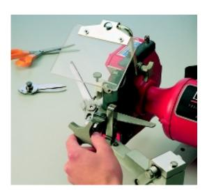
With the patented, rotating blade clamping system blades are clamped just once to grind, steel and buff the entire blade edge. Even curved blades and blades up to 16".
