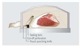
The **pouch punching knives** are necessary so that the package can be evacuated even if the bag opening protrudes from the chamber.
