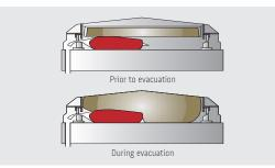
The **expansion cushion** with **removable frame** reduces the evacuation time by up to 30% and prevents folds on the top side of the package.
