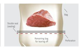
The **cut-off perforation** allows easy removal of protruding bag material after removal of the packages.
