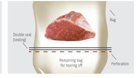
The **cut-off perforation** allows easy removal of protruding bag material after removal of the packages.
