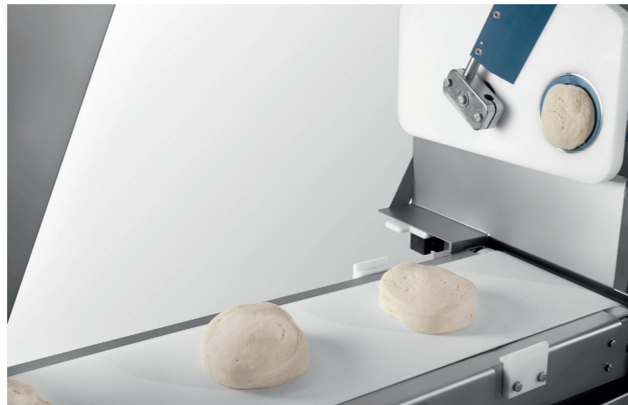
Rotating portioning scraper
