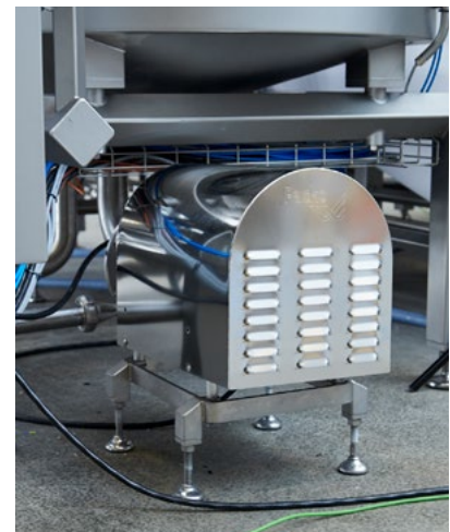
Pumps are positioned/mounted on own frame for easy access at inspection/maintenance, etc. In addition, the pump of the scanGravy mixing unit can be equipped with its own knife system for eliminating lumps in "challenging to produce" gravies.
