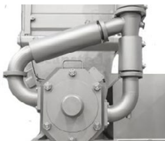
SuperPump SP 290 showing double pump discharge.
