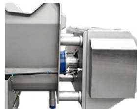
Please also note drain/cleaning built-in drain plug.
