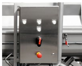
Standard screw conveyor electrical/operator panel.
