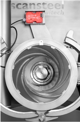
Cabinet without worm showing the flights of the lining.
