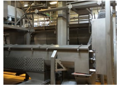
scansteel foodtech Whole Pallet Crusher, WPC 2000-Single, shown in application where existing footprint is sparse and where the pre-broken frozen blocks need to be elevated to approx. 5000 mm.
