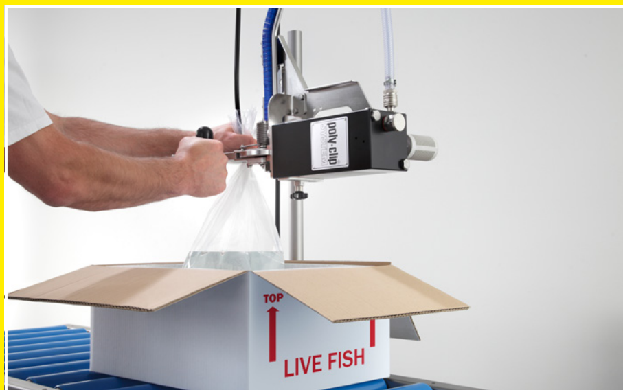
After filling with oxygen, the gate is closed and the clipping process is thus triggered.
