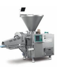
The dough divider with integrated cutting device and conveyor has been developed to divide doughs with a great wheat content: The VEMAG systems score thanks to their high output performance - up to 9,600 portions per hour for example for sandwich bread doughs. Since work is managed without the aid of oil, the dough divider works very economically.
