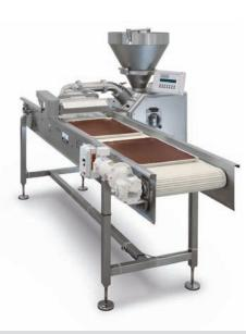
The sheeting horn is used in all applications where soft doughs and mixtures are divided to an exact weight and are positioned directly onto sheets or sheet-form products such as tray-bakes, toppings, fillings or brownies. The sheeting horn is fitted with a pneumatically operated roller closure and can be adjusted to the specific requirements such as different sheet sizes.
