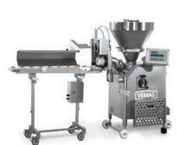
Perfect for weight exact dividing of doughs and the output of small bakery items such as cookies, cereal bars, biscuits or muffins. Versatile in its use also with conveyor flouring or oiling system for soft doughs. The dough dividers can be reconfigured within minutes - e.g. with a sheeting horn for traybakes or filling heads for mixtures. The R500 is the smallest in the family of VEMAG dough dividers.
