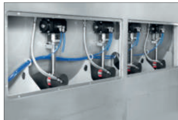
Cooling valves and nozzles behind the cover
