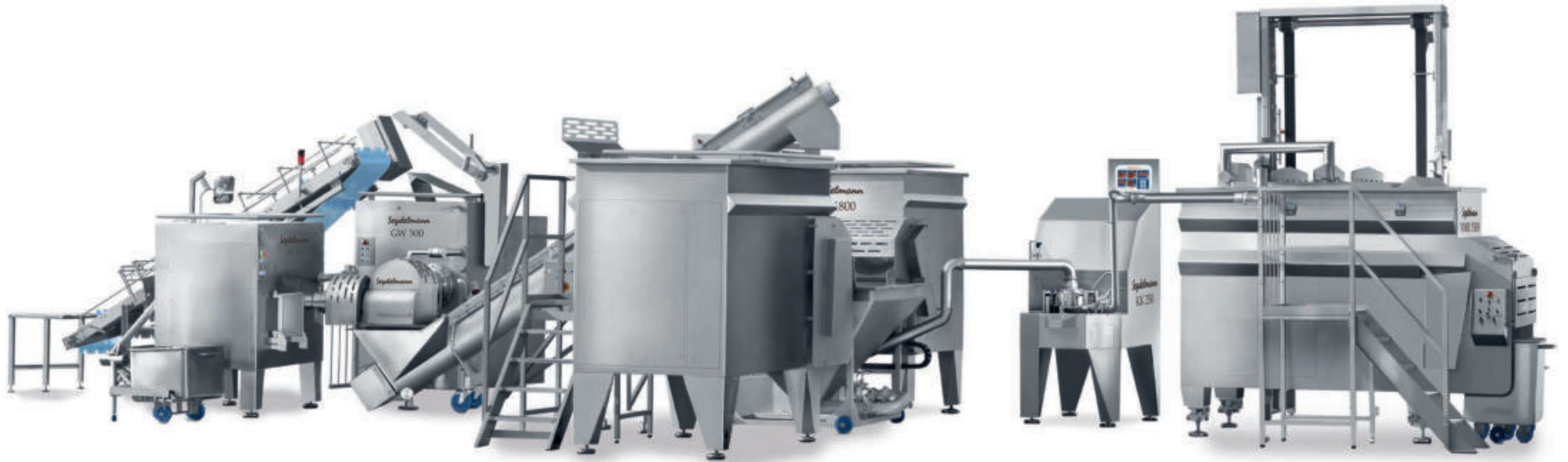
Production Line with Automatic Grinder AG 160, Frozen Meat Grinder GW 300, swiveling screw conveyor, two Mixers MR 1800, 1200 l hopper with pump and tube connection, Konti-Kutter KK 250 AC-6 and Vacuum-Mixer VMR 3500 with loading device for large containers
