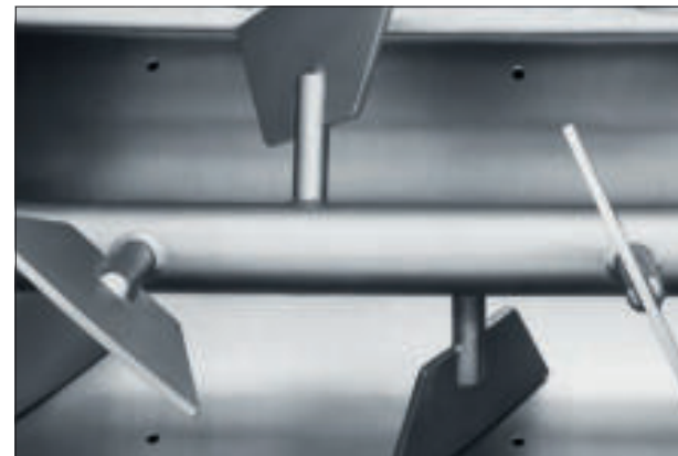
Mixer with mixing paddles and cooling nozzles
