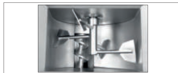
Mixing unit above the working worm
