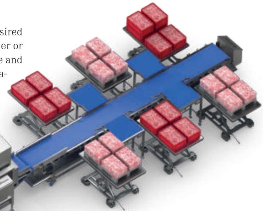
Weighing feeding belt with scissor lifting tables and X-ray fat analysis, inclined conveyor belt with flights, Universal Grinder AW 300 U, swivelling screw conveyor and three Automatic Mixer Grinders AMR 2500 with liquid gas cooling.
