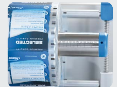
Open design, ergonomic access: the Amax-series traysealers simplify cleaning, maintenance and service.
