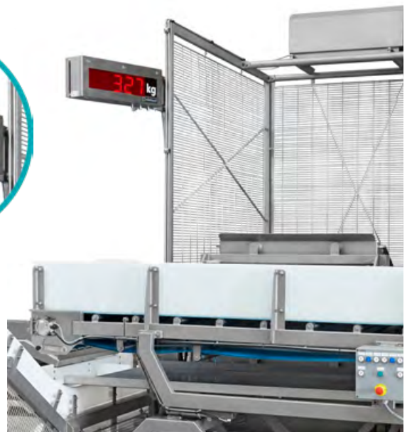
Details showing drip trays and weighing/load cells.
