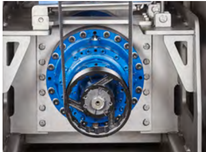
Planetary gear box assembly. Between gear box and crusher claw, a Heavy Duty clutch system prevents damage to the gear box in case a large foreign (metal) object by mistake is thrown into the Whole Pallet Crusher.
