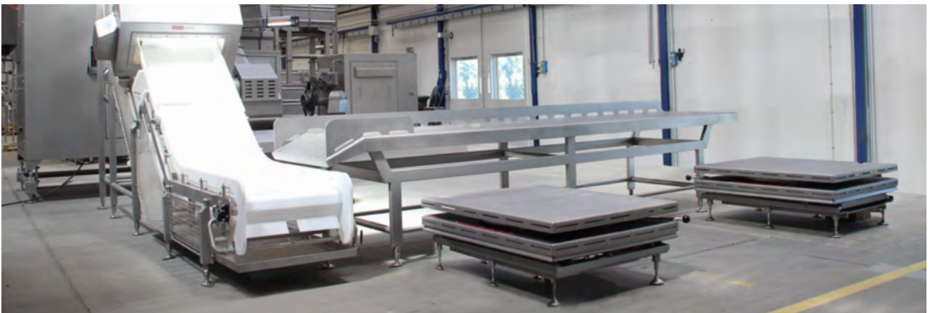
Unpacking station with 2 (two) lifting tables for ergonomics, left side.
