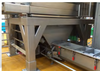
Horizontal screw shown with closed lid.
