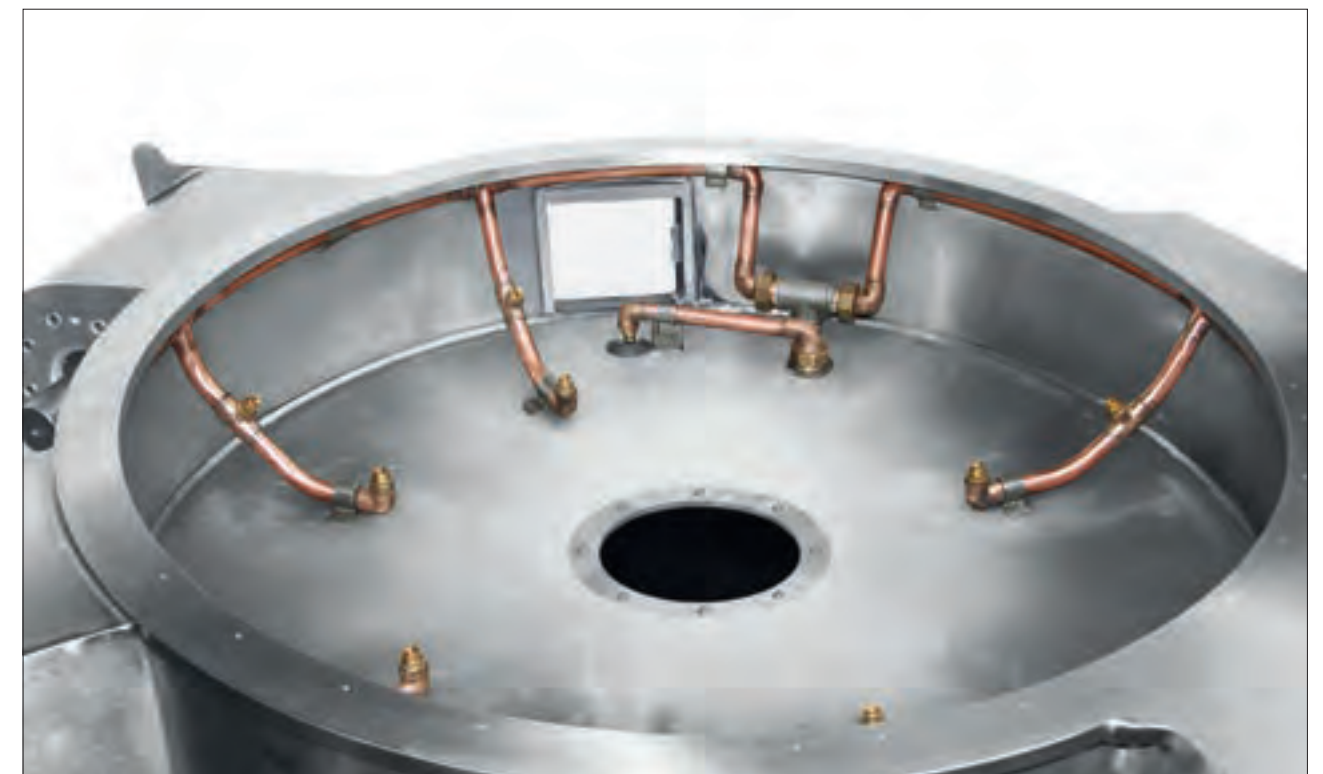
Nozzle system Cooking-Cutter (optional stainless steel loop)
