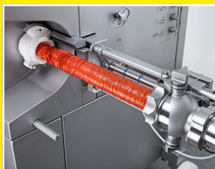
Safety casing brake with hand guard
