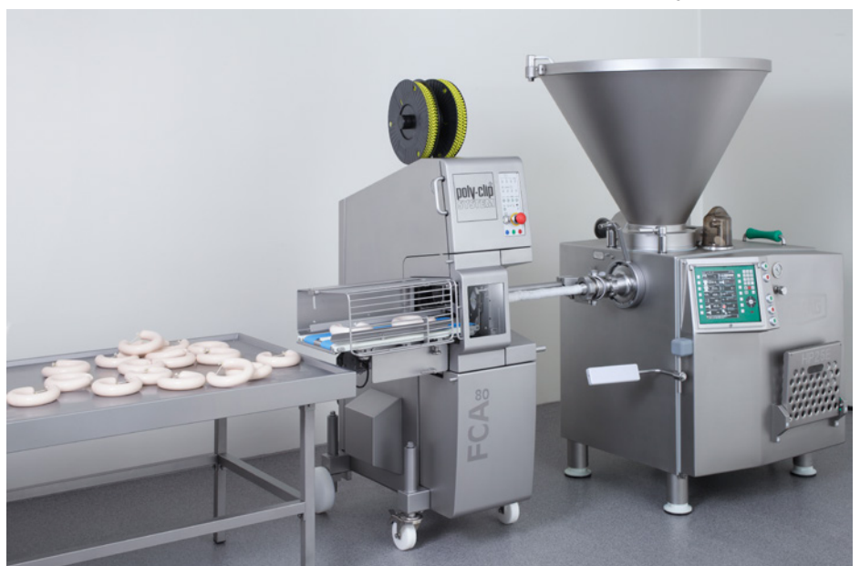
FCA 80 with adjusted front flap and double-conveyor belt specifically for rings
