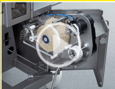
Retractable automatic loopers GSA for easy reloading of loops
