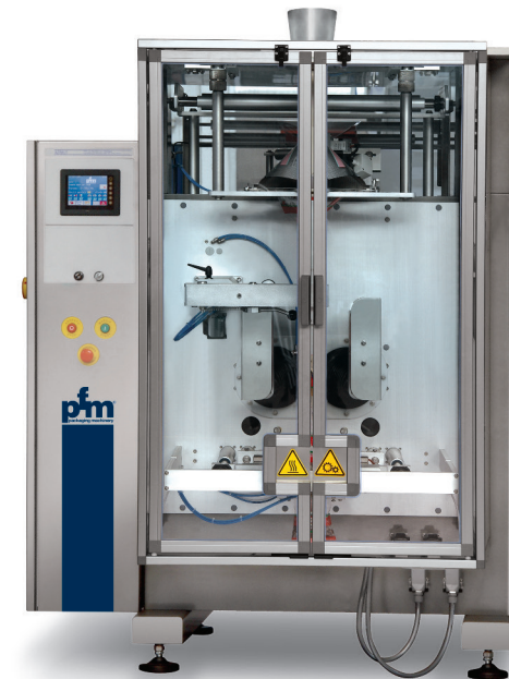
VFFS wrapper mod. Azimuth to obtain Steelo-bags with lid application
