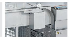
**Cut-off device**By means of rotary blades, protruding bag material is cut off in front of the chamber.
