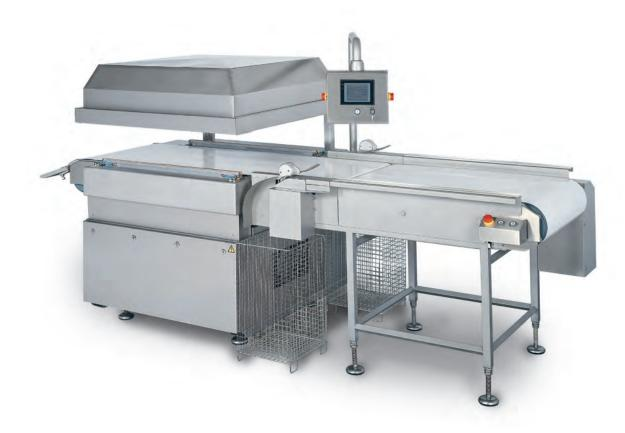
Constructed of corrosion-resistant stainless steel. Easy-to-clean, hygiene-friendly machine design.
