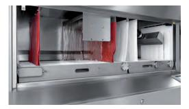
Left – two water curtains from above and one water nozzle from below.
