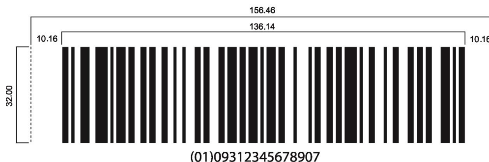
Figure 1: GTIN-13 with a filler zero encoded in a GS1-128 barcode
