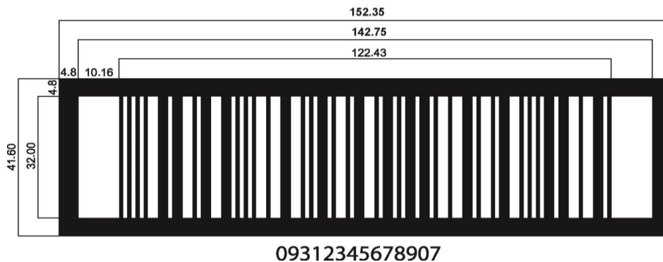
Figure 2: GTIN-13 with a filler zero encoded in an ITF-14 barcode
