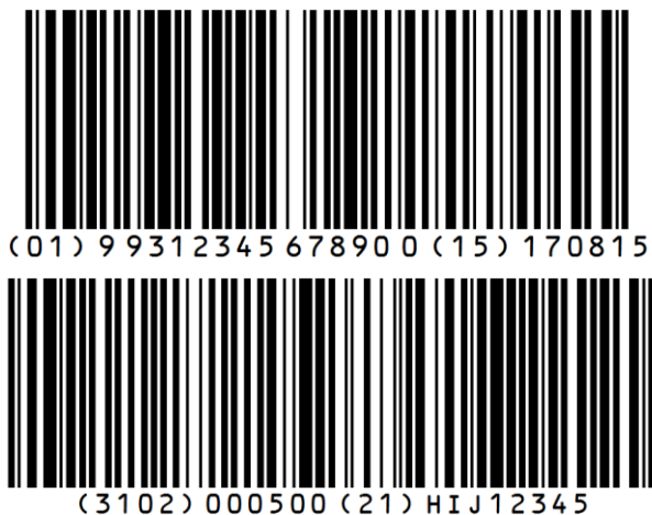
Figure 5: Encoding GTIN, Best Before Date, Net Weight and Serial Number in a stacked barcode
