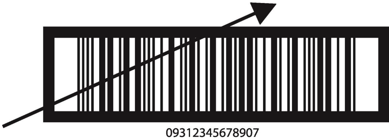
Figure 2: Example of a Skewed Scanning Beam
