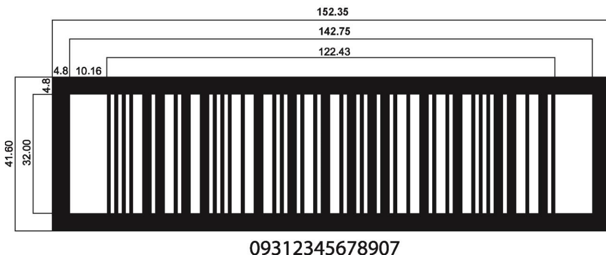
Figure 1: Measurements of a GTIN-13 with a filler zero encoded in an ITF-14 barcode at an X-dimension of 1.02 mm
