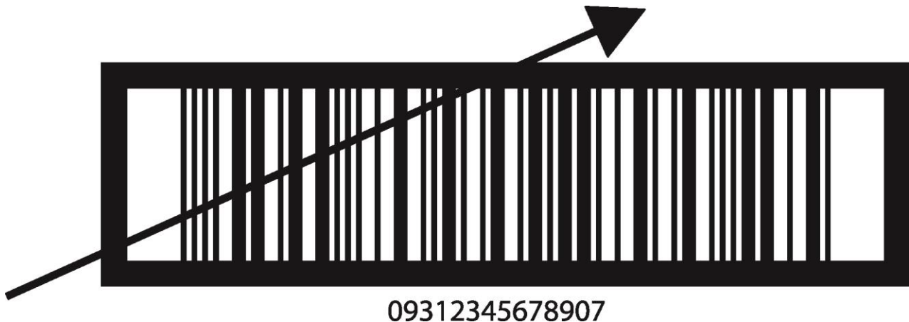
Figure 2: Example of a Skewed Scanning Beam
