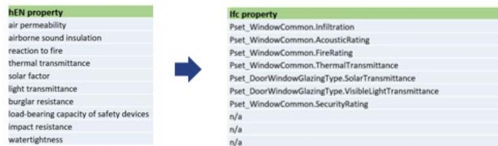
*Illustration: Standardised properties vs. IFC Properties. Cobuilder AS @ 1997-2019*
