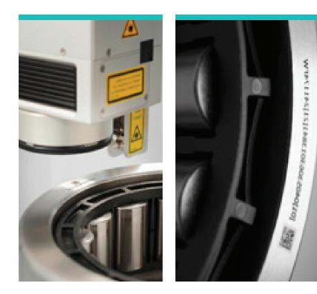
HFG uses laser technology to etch each DataMatrix barcode onto its respective system or component so that it can always be accurately identified throughout its entire lifecycle. Now with a single scan, all stakeholders—whether HFG, railway operator, MRO workshop or testing/certification organisation—can easily identify the bearing and access all associated information to track and trace its location and path along the supply chain and support MRO services on a customer's site.
