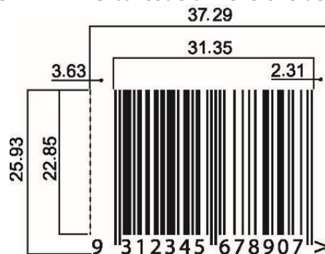
Figure 1: EAN-13 barcode dimensions at nominal size (100%)
