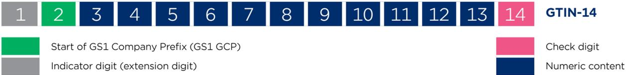
If you are using SGTIN, AI (Application Identifier) 21 is used to encode the serial number. This is explained in chapter 4.1. Serial number cannot exceed 20 digits/alphanumeric characters.
