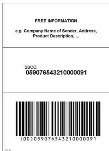
Figure 6: Example of a GS1 Logistic Label for a logistic unit with different items.
