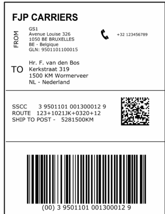
Figure 3: Example of a GS1 Logistic Label for a parcel (including a GS1 DataMatrix barcode)
