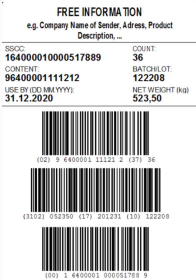
Figure 2: Example of a GS1 Logistic Label for a logistic unit with variable measure items
