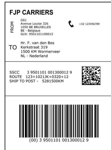
Figure 7: Example of a GS1 Logistic Label for a parcel (including a GS1 DataMatrix barcode)
