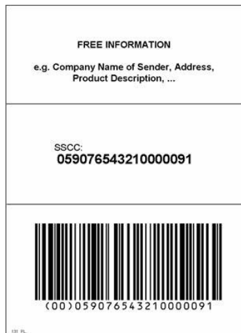
Figure 6: Example of a GS1 Logistic Label for a logistic unit with different items.
